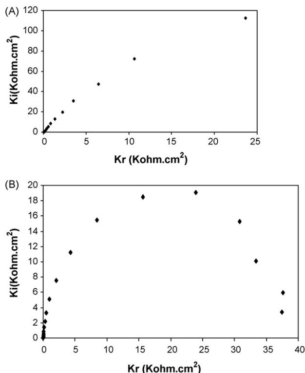
Fig. 6. Nyquist plot for (A) Al<sub>2</sub>O<sub>3</sub>/sonogel-carbon electrode and (B) AChE/Al<sub>2</sub>O<sub>3</sub>/sonogel-carbon electrode.
