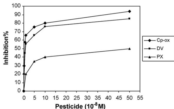
Fig. 5. Inhibition curve of AChE immobilized in Al<sub>2</sub>O<sub>3</sub> sol-gel matrix by paraoxon (Px), dichlorvos (DV) and chlorpyrifos-ethyl-oxon (Cp-ox), 10 min incubation. Measurement conditions: 0.2 M phosphate buffer, pH 7.0, applied potential: 210 mV, 1 mM acetylthiocholine substrate concentration.
