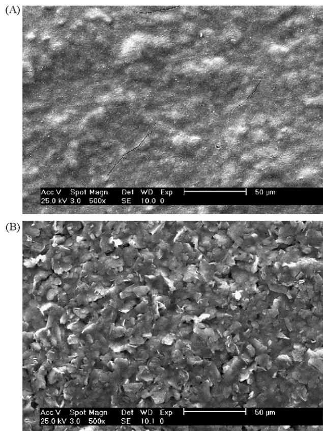
Fig. 7. Scanning electron micrograph of (A) Al<sub>2</sub>O<sub>3</sub> sol-gel/sonogel-carbon electrode and (B) AChE/Al<sub>2</sub>O<sub>3</sub> sol-gel/sonogel-carbon electrode, obtained at 25.0 kV with a 500 $\times$  zoom.
