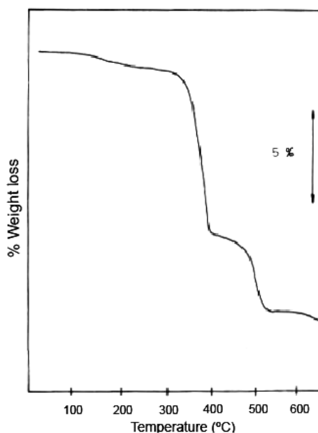
Figure 9. TGA diagram of a sample of \text{La}(\text{OH})_3 . Adapted from [17].
