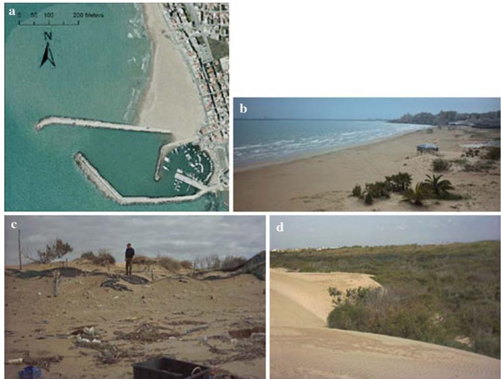
Grande breakwater, 60,000 m<sup>2</sup> and 21,000 m<sup>2</sup> of new beach were respectively formed in the 1967–1977 and 1977–1987 periods. At Santa Maria del Focallo, the beach eroded and this was evidenced by undermining processes at the littoral road (which was protected by concrete blocks, Fig. 7c), dune escarpments and vegetal dune cover degradation.
