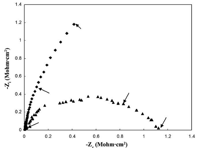
**Fig. 3.** Nyquist plots for impedance data obtained at 0 V for unmodified Sonogel-Carbon electrodes (▲) and 5%  $\beta$ -CD-Sonogel-Carbon electrodes (◆). Frequency range: 100 kHz–10 mHz.
