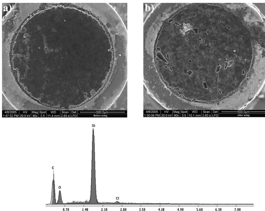
**Fig. 5.** Micrographs corresponding to the 5%  $\beta$ -CD-Sonogel-Carbon electrode polished: (a) before using, and (b) after using. The EDS spectrum corresponding to both micrographs is also included.
