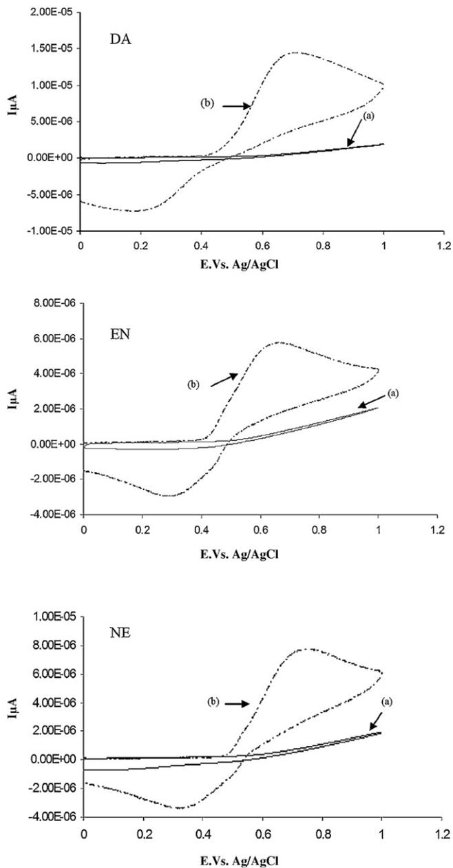
**Fig. 2.** Cyclic voltammograms for 5 mM of D,L-norepinephrine (1), epinephrine (2), and dopamine (3) at: (a) an unmodified Sonogel-Carbon electrode, and (b) a 5%  $\beta$ -CD-Sonogel-Carbon electrode; scan rate = 50  $\text{mV s}^{-1}$ ; PBS buffer at pH 7.4.
