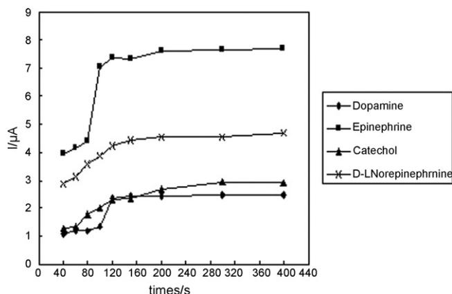
Fig. 1. Effect of the accumulation time on the peak height for  $5 \times 10^{-4}$  M of epinephrine, dopamine, D,L-norepinephrine and catechol in PBS buffer at pH 7.4 using a 5%  $\beta$ -CD-Sonogel-Carbon electrode.
