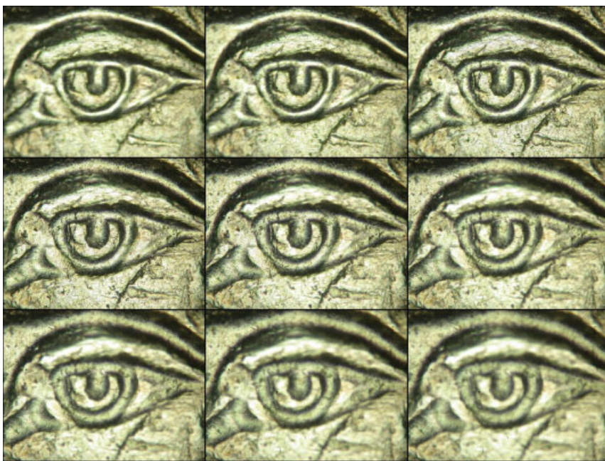
Fig. 6. Representative composition with some of the 19 images taken of a real sample (1 euro coin), using an optical microscope. All the images were captured using the same photographic conditions; resolution ( 640 \times 480 ), focal distance (14 mm), aperture ( f/3.3 ) and exposition (1/125s). [Color figure can be viewed in the online issue, which is available at www.interscience.wiley.com .]
