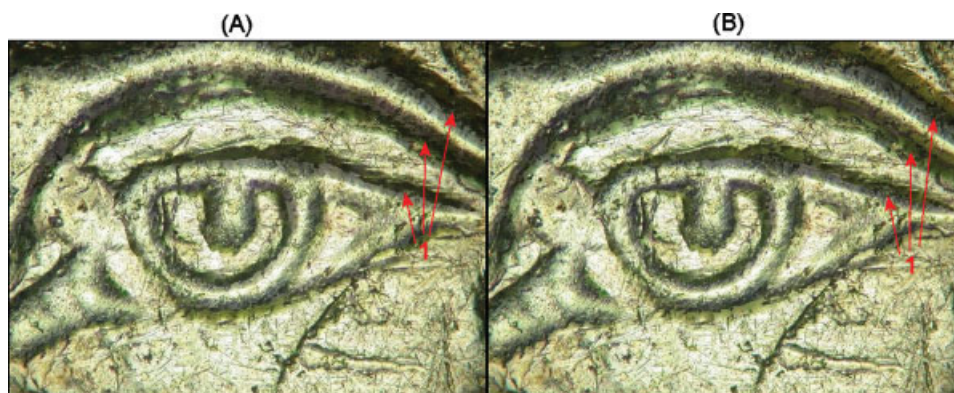
Fig. 7. Extended depth of field image obtained by applying the algorithm to the 19 real images of a coin obtained with a high magnification microscope. (A) using the RGL variables, which have the highest second variance values, as the basis for the calculation, and (B) using the L variable. [Color figure can be viewed in the online issue, which is available at www.interscience.wiley.com .]
