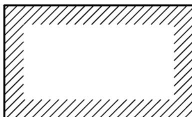
Figure 4 — Hatched contour of large area
