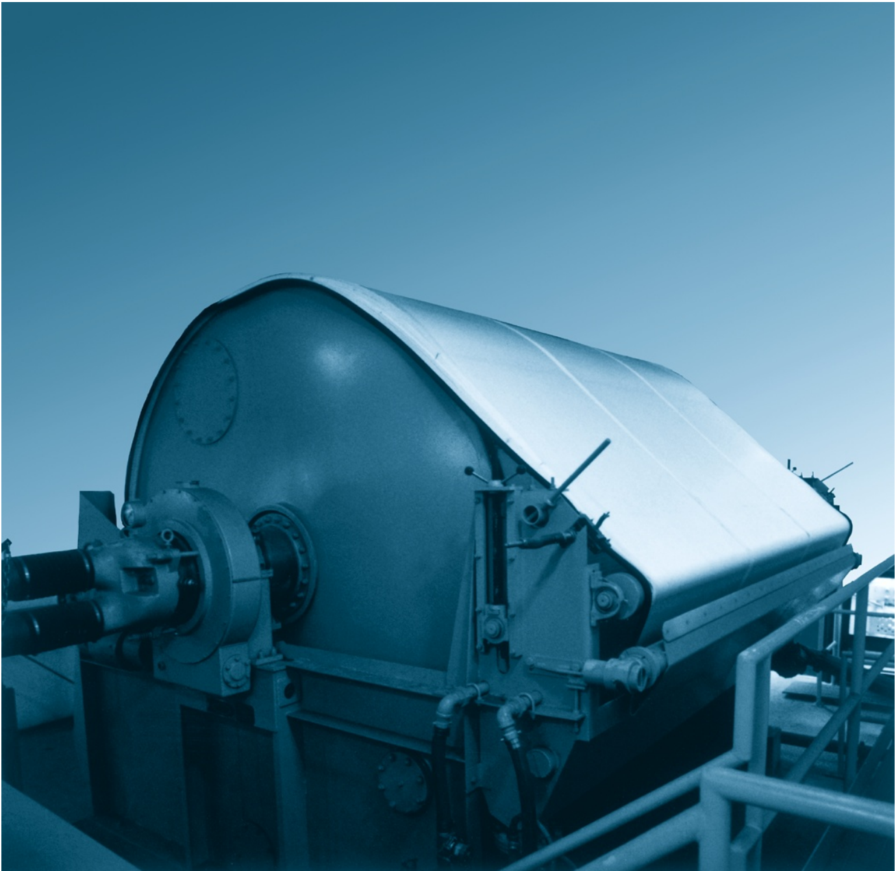
GL&V/Dorr-Oliver 8 x 10 ft. Drum Filter with Belt Discharge
