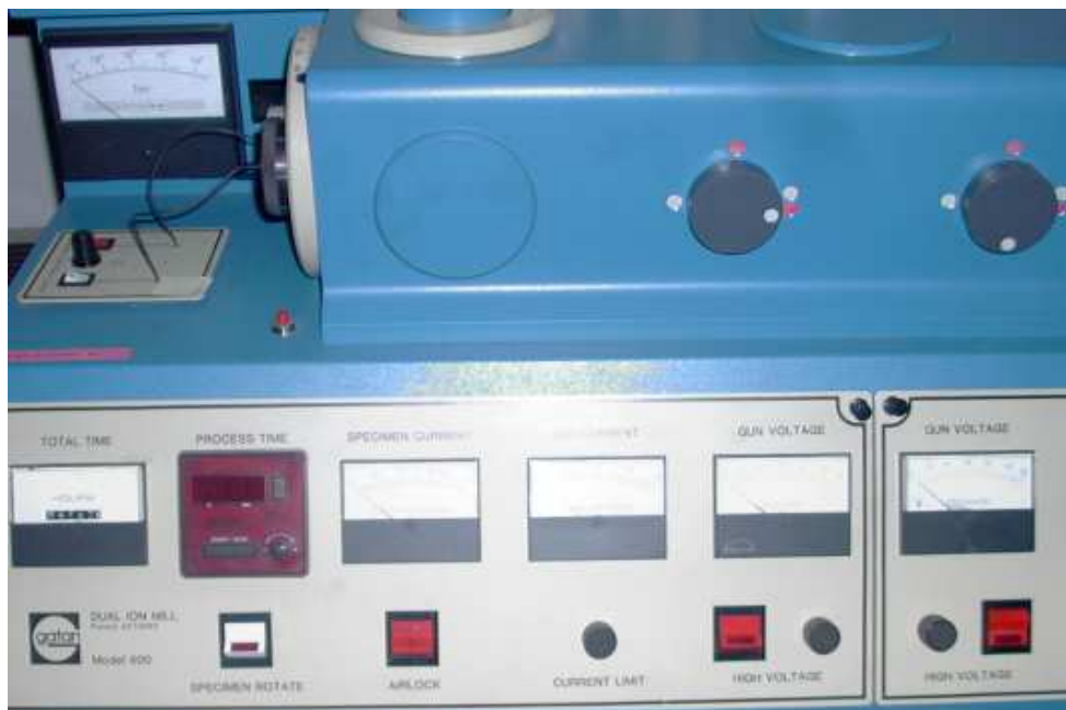
Panel de control de "Ion Mill"
