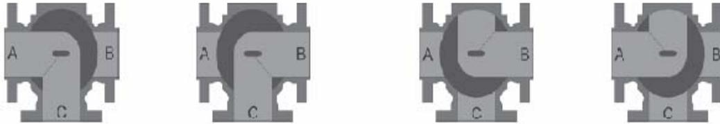
Fig. 6 - Flow schematics of Type BR 26t Three-way Ball Valve with horizontal "T" port
