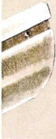
Sterntube bearings are available in standard sizes or to customer drawings and specifications. High tin or high lead based white metal is centrifugally cast into the bearing shells which are specially treated to ensure a metallurgical bond strength of at least 4000N/cm<sup>2</sup>. The bearing shells are de-graphited using the well tried and tested Kolene
