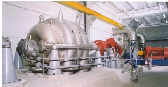
RC blowers, as shown, may be installed as single unit or in tandem arrangement.
