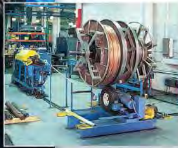
Use of rolled coil tubing supports the flexibility inherent in DFT manufacturing. Special straightening equipment and unique burr-free cutting process result in superior rolled joints.
