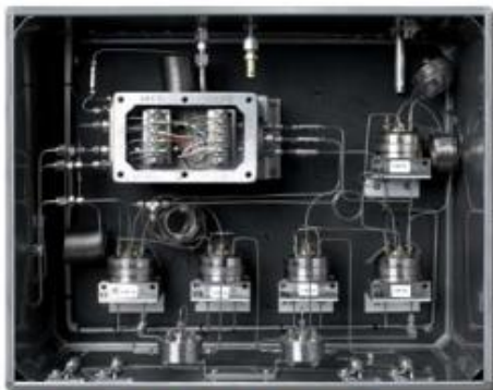
The air bath oven design of the Model 1000A Process Gas Chromatograph offers maximum analytical flexibility while maintaining easy access to all analytical components.
