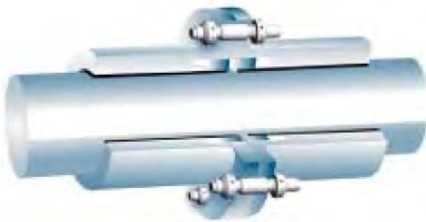
Flange couplings and Supergrip bolts combination for limited space
